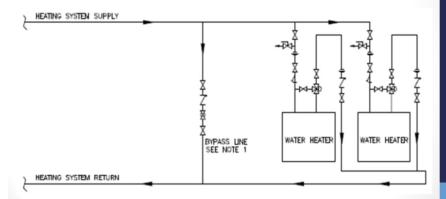
Note: Size bypass line to ensure that RWT to non-condensing, high mass boilers always remains above 140°F
