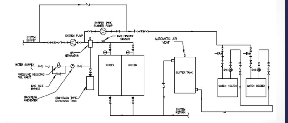
For use when DHW is the only load on the system (spring/summer) Allows for main system pump shut down
